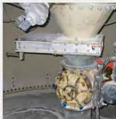
12" (305mm) Maintenance Gate above a rotary airlock handling soda ash
