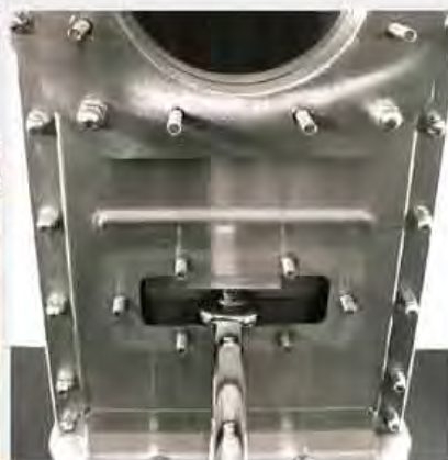
Blade adjustment through front access panel
