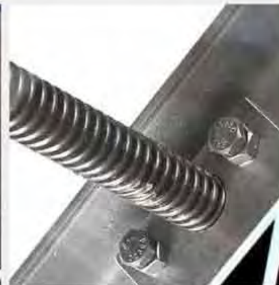
Ratio of 5:1 ACME threaded rod provides the ability to cut through a column of material in an upset condition
