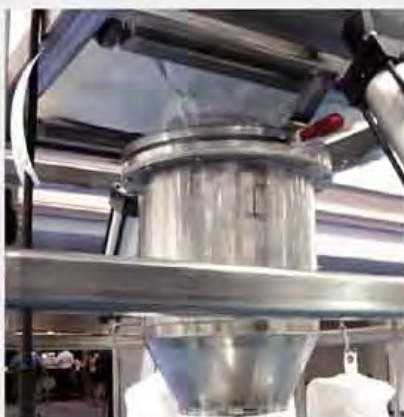
18" (457mm) Iris Valve on bulk bag discharge
