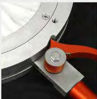
Preset positions for quick adjustments of material flow
