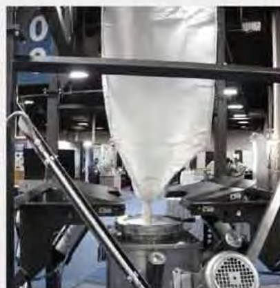
15" (381mm) Iris Valve on bulk bag discharge
