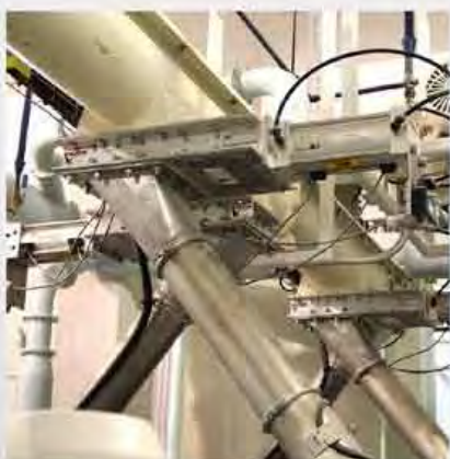
13" (330mm) Roller Gate below a screw conveyor
