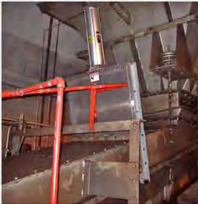
24" x 38" (610mm x 965mm) Aggregate Gate mounted within a vibratory feeder metering the flow of coal
