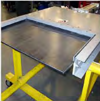
24" x 38" (610mm x 965mm) Aggregate Gate mounted within a vibratory feeder metering the flow of coal
