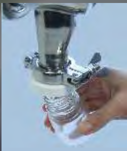
PTFE Bottle Adapter - the sample collecting bottle screws into bottle adapter
