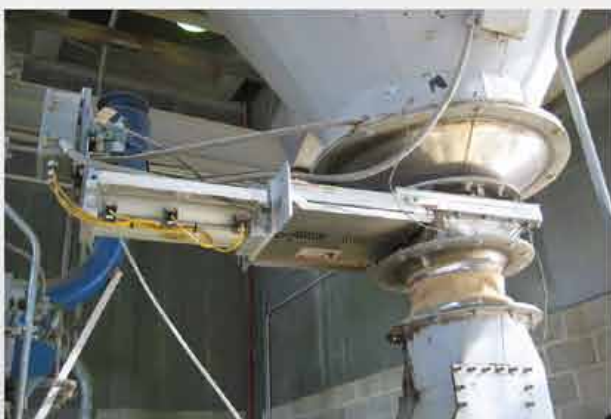
10" (254mm) Clear Action Gate below hopper handling animal feed additives
