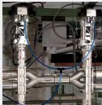
2.5" (63mm) Wye Line Diverter handling dry leaf tea
