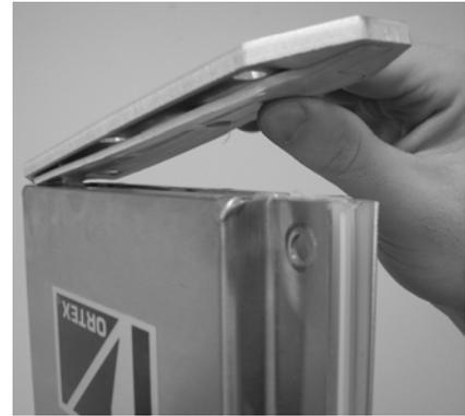
It is recommended the gate be bench tested before returning it to service. For test purposes only, the gate should operate smoothly at approximately 2.5 barg. Shim may need to be added or subtracted. A minimum of 5 barg is needed when the valve is returned to system operation.
