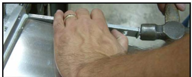
17) Work the material all the way around the Seal Retainer Groove. Cut the Packing Material at a 45° angle, allowing a slight material overlap.
