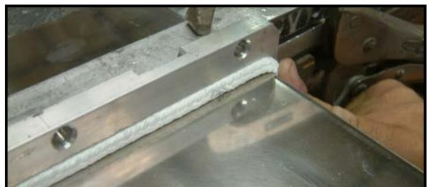
15) Utilizing a small piece of aluminum bar and a hammer, "tap" the Packing Material into the groove around the corner of the blade.
