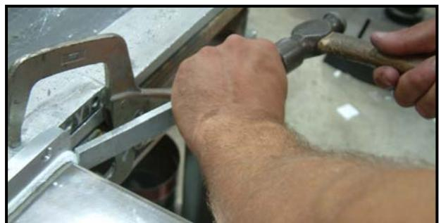
16) Make sure there is a "snug" fit on the top, side, and bottom. Be careful not to scratch or damage the blade.
