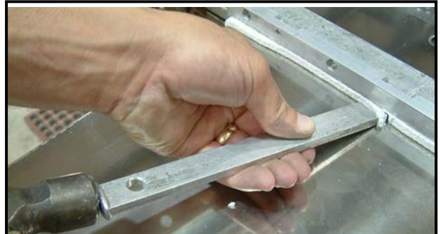
20) Utilizing aluminum bar, make sure material is snug around the top, side, and bottom of the Blade edge.
