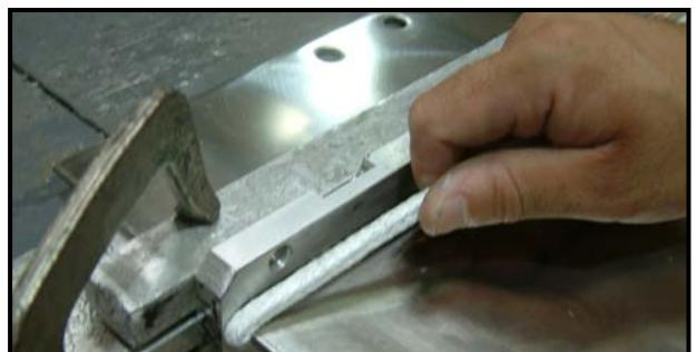
19) Utilizing aluminum bar, tap material into groove on top and bottom of blade.
