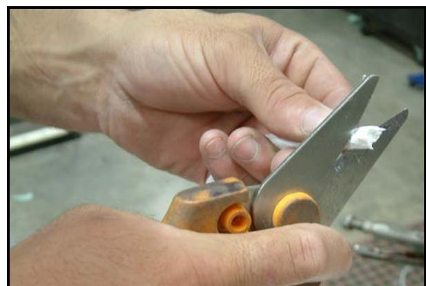
12) The Braided Teflon Seal Packing Material is configured in a slight rectangle. Holding the material lengthwise, cut one end of the material at a 45° angle
