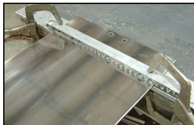
10) Utilizing two softer pieces of metal (e.g. aluminum), and taking care not to scratch the blade, clamp the blade to the end of a workbench. (Note placement of clevis mounting holes.)
