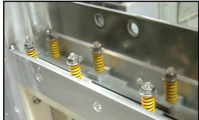
8) Remove the Seal Retainer Bar.
