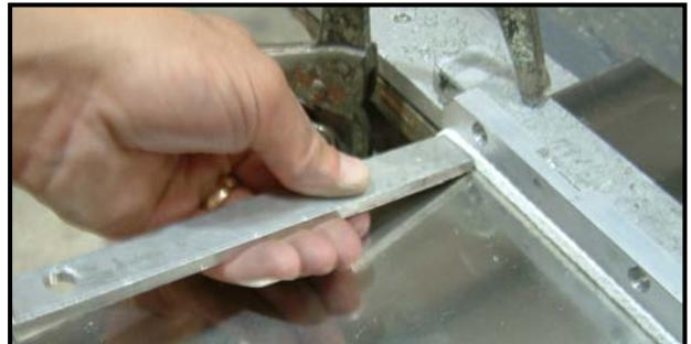
21) Unclamp Blade and Seal Retainer Bar from workbench and carefully slide it into Maintenance Gate frame.
