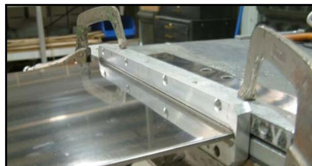
11) Slide Seal Retainer Bar onto blade.
