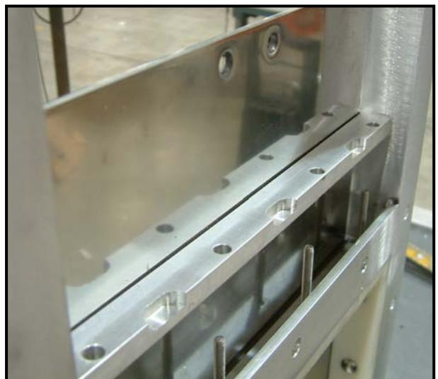
22) Reverse the procedures from step 7 to reassemble the gate. (When tightening the Nuts holding the Pressure Springs, alternately tighten Nuts on either side of the Blade that are not directly opposite each other.)
