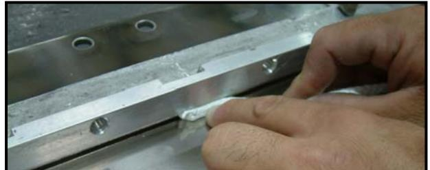
14) Form the material around the edge of the blade and continue on the underneath side.
